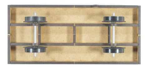
Place the axles through the bearings in the sole bars, then push on the wheels with a flange to flange distance of 28mm, there will be approximately 5mm of the axle projecting from the outside of each wheel this is OK and it does not need to be trimmed off.
