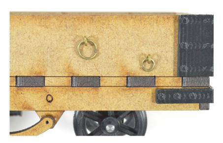
Fit them as shown with the 4 smaller rings at either end of each side and with the larger ring on the same side as the brake handle.
